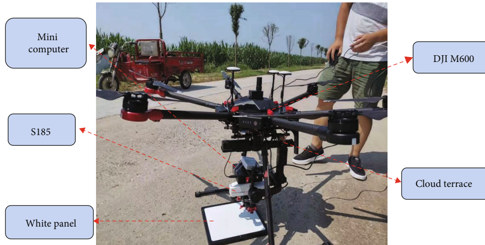
FIGURE 2: UAV-based hyperspectral imaging system.
